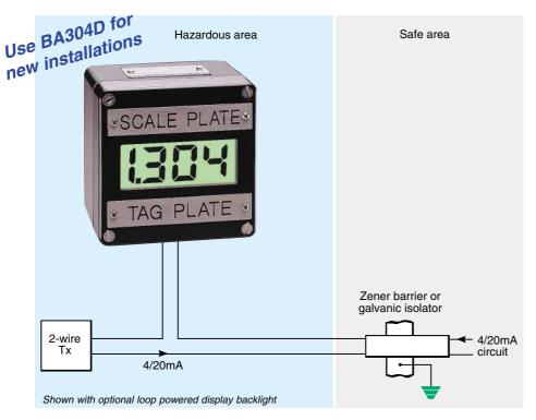
The BA304C is an intrinsically safe field mounting indicator which displays the current flowing in a 4/20mA process loop in meaningful engineering units. The indicator has a 25mm high, easy to read liquid crystal display, and is housed in a robust IP66 enclosure. Modular accessories enable only the required features to be incorporated, thus reducing cost while retaining interchangeability between instruments.
